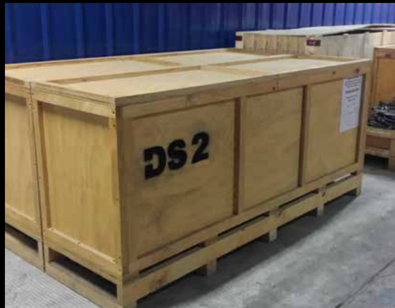
Typical packaging for the shelter kit, Crate dimensions are 2.5m L x 1.1m T x 0.8m W. Each crate weighs approximately 300kg.
