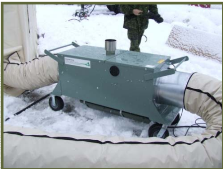
Special military designed air heaters with remote thermostat and CO detector plus non-mercury tip-over sensor. Military quick disconnect skid kit is available.
